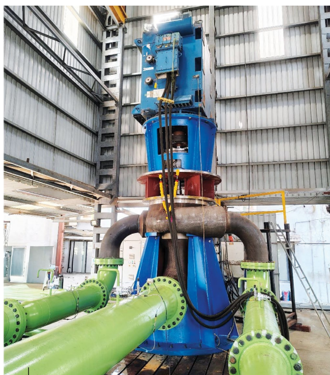
Indigenously designed and developed Primary Coolant Pump (PCP) for 700 MWe Pressurised Heavy Water Reactor (PHWR)
